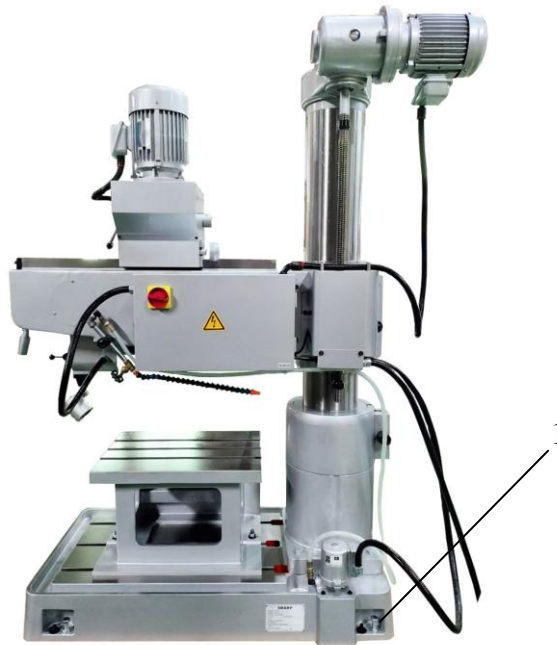
1. The level adjusting bolts.
