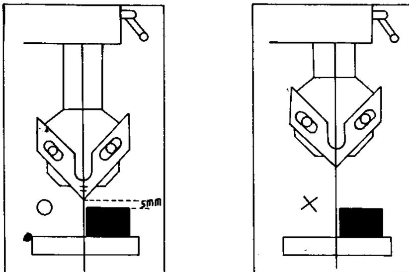
**5. In operating, blade should be in the middle of the Blade Guide exactly to prevent wear of the Blade Guide. °**
