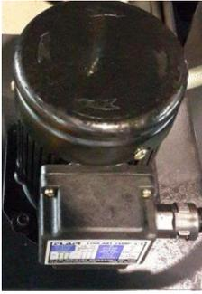
When the hydraulic system is turned on, the coolant pump can be operated individually from the control panel. Coolant can be used to wash off chips as well as providing cooling during cutting.
