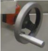
This device is used to preset the required cutting length of a workpiece for automatic cutting. When the handwheel is turned clockwise, the cutting length of the workpiece is shortened. When the handwheel is turned counterclockwise, the cutting length of the workpiece is lengthened.
