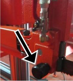
Step 9 - Open the wire brush cover. Loosen the lock lever and lower the wire brush.
