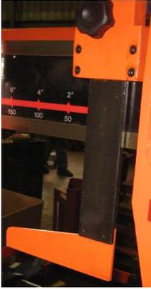
This device allows the blade to quickly descend to just right above the material to save you operation time.
