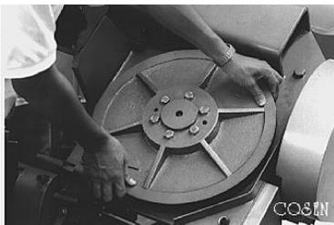
Step 14 - Make sure the back of the blade is also pressed against the flange of the idle wheel.
