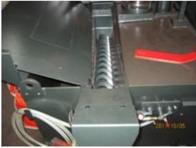
Chip conveyor is a spiral device to bring chips out during cutting.
