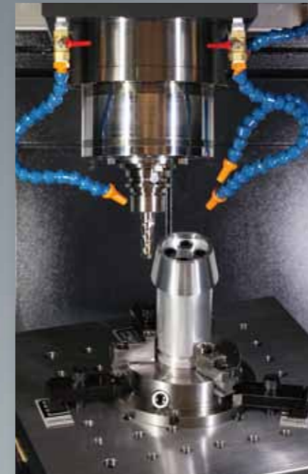
Taper cone cutting test
