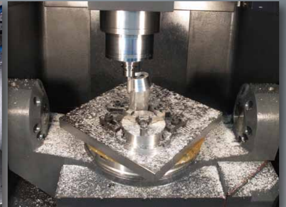
Taper cone cutting test
