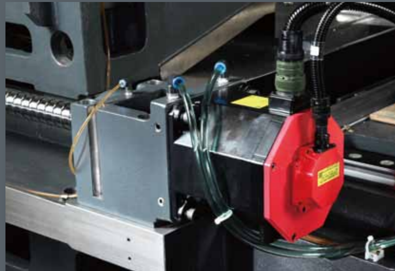
ballscrew bracket cooling feature
