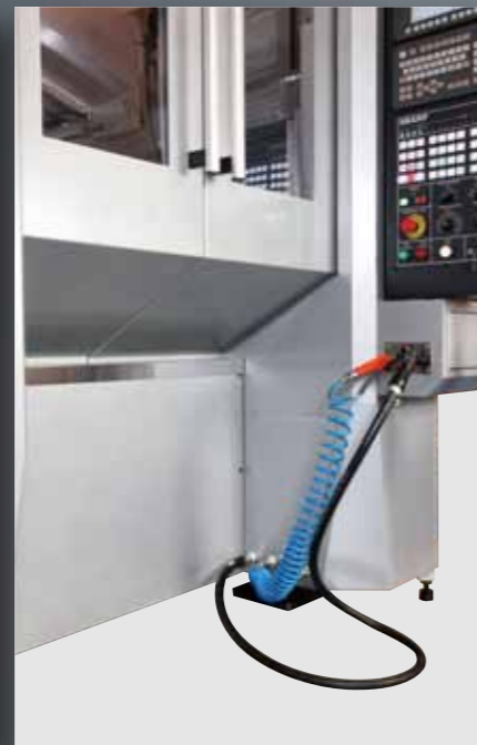
Front mounted coolant gun and air gun
