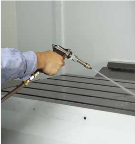
A convenient hand held coolant nozzle is provided for washing the work piece and the inside of the machine enclosure.
