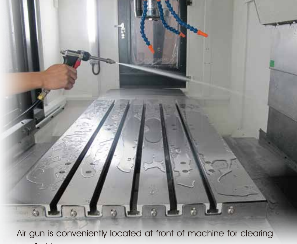
A convenient hand held coolant nozzle is provided for washing the work piece and the inside of the machine enclosure.
