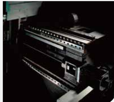
TRIPLE GUIDEWAYS FOR Y AXIS MOVEMENT ▶ 2 roller type linear guideways are on the face of bridge, and the 3rd is located on the top to offer excellent holding of headstock.
