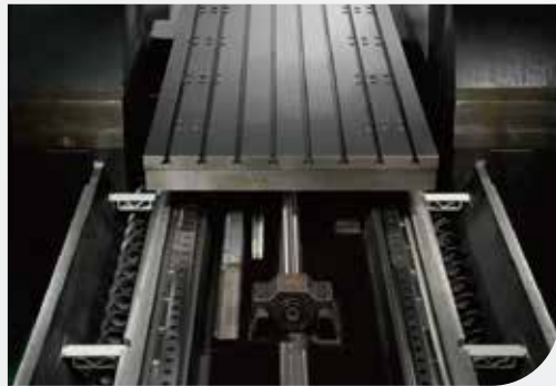
LARGE PRELOADED HIGH PRECISION BALLSCREWS ▶ Double nut C3 class precision ball screws are used on all three axes. ▶ Direct drive from servo motor to ball screw. ▶ Ball screws diameter: X:63mm / Y: 40mm / Z: 50mm. ▶ Rapid traverse speed X,Y: 1181 ipm (30M/min), Z: 630 ipm (16M/min) ▶ Table size :86.6" x 40" (2200 x 1100 mm) ▶ Maximum table load : 6,600 lbs (3,000 kg) ▶ One-piece base with two slots for chip auger at both sides minimizes cleaning time.
