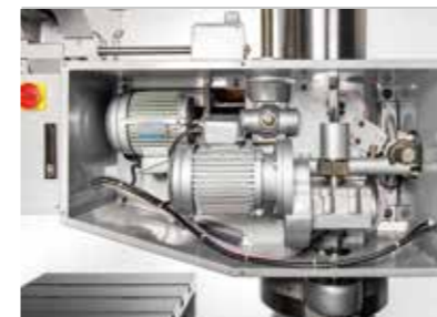
Model RD-1230 Electric motor elevating arm with separate motor for clamping.
