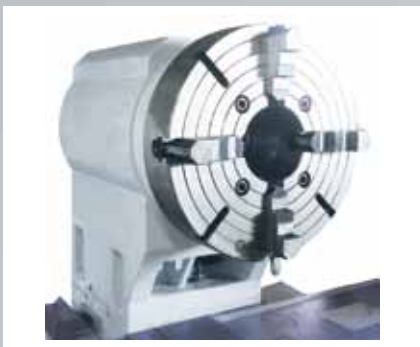
Customized tailstock with chuck
